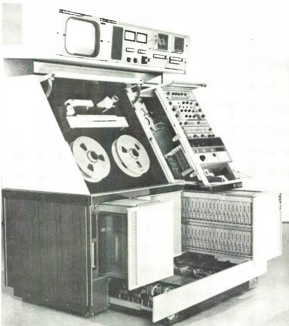
Fig. 5 Access to the electronics is facilitated by the roll out sections.
